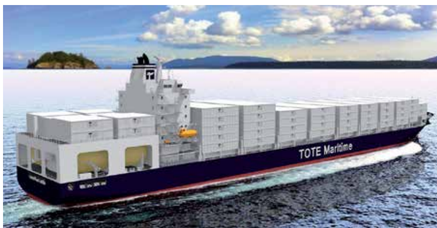
Fig. 2: New TOTE container vessel powered by MAN B&W dual fuel ME-GI
