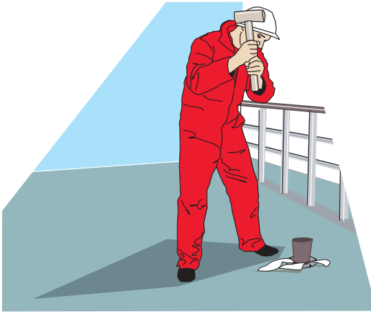
Block all deck scuppers
