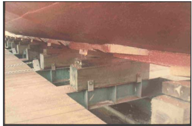
TIMBER CRUSHED AT NARROW KEEL
