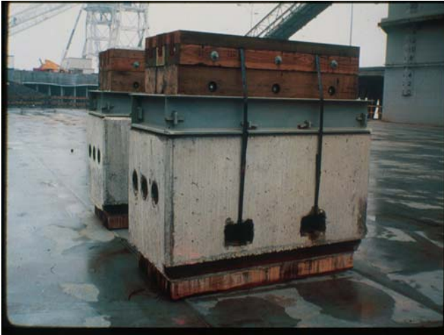
Concrete/timber Composite Block
