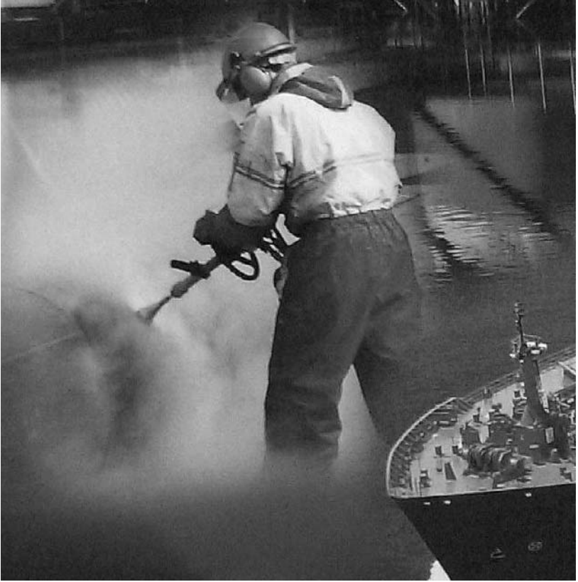
Figure 3 Hull preparation by water blasting and hull painting by airless spray
