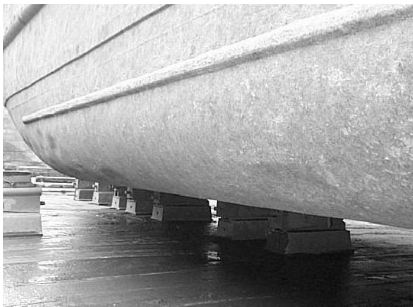
Figure 1 A vessel sitting on keel blocks undergoing repairs in dry dock
